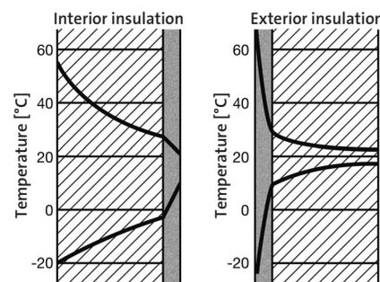
2 The temperature profile shows that the exterior wall remains colder in the winter through interior insulation
