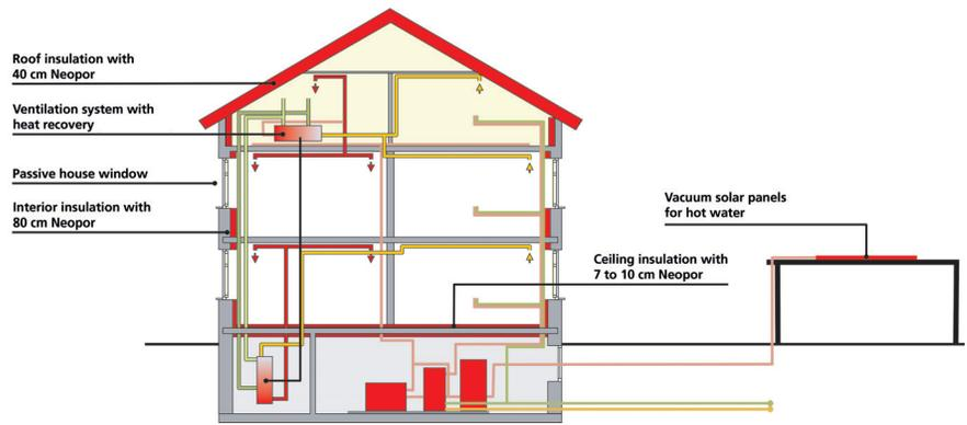
4 Walls, roof and cellar ceiling were insulated with insulating materials of Neopor, a silver-grey, graphite-bearing EPS.
